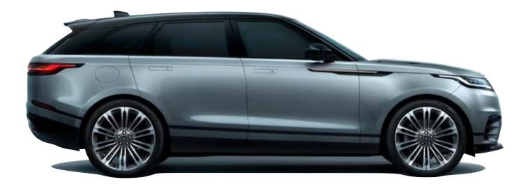
Width 2,041mm mirrors folded Width 2,147mm mirrors out
